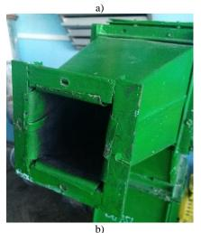
Fig. 1. Experimental installation: a) – nozzle №1 for a swirl air jet; b) – nozzle №2 for a compact air jet
