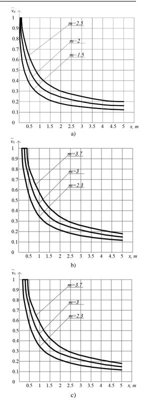
Fig. 4. Dependencies of the different air jets axial dimension-less velocities at the different angles  $\beta$  ( $\beta = 0^{\circ}, 45^{\circ}, 90^{\circ}$ ) of change of a flow direction from the current coordinate *x*: a) flat air jet; b) rectangular air jet; c) compact air jet.
