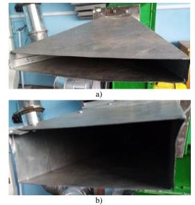
Fig. 2. Experimental installation: a) – nozzle №3 for a flat air jet; b) – nozzle №4 for a rectangular air jet
