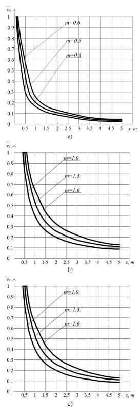
Fig. 3. Dependencies of the swirl air jet axial dimensionless velocities at the different angles β (β = 0°, 45°, 90°) of change of a flow direction and twisting plates inclination α from the current coordinate *x*:
